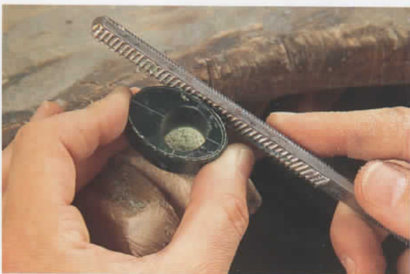
5 I used a coarse four-in-one file to roughly shape the wax ring.
