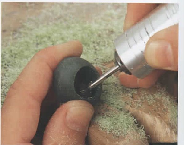
8 The interior of the wax ring was hollowed out with a wax ball bur attached to a flexible shaft.
