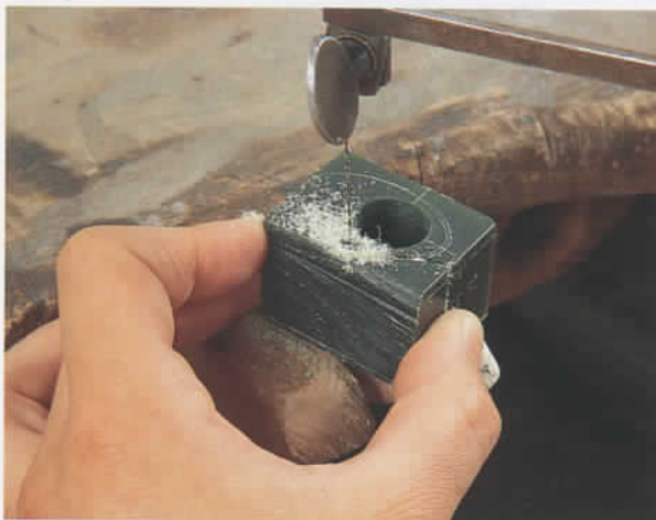
4 A spiral blade was used to saw the wax into a ring shape.
