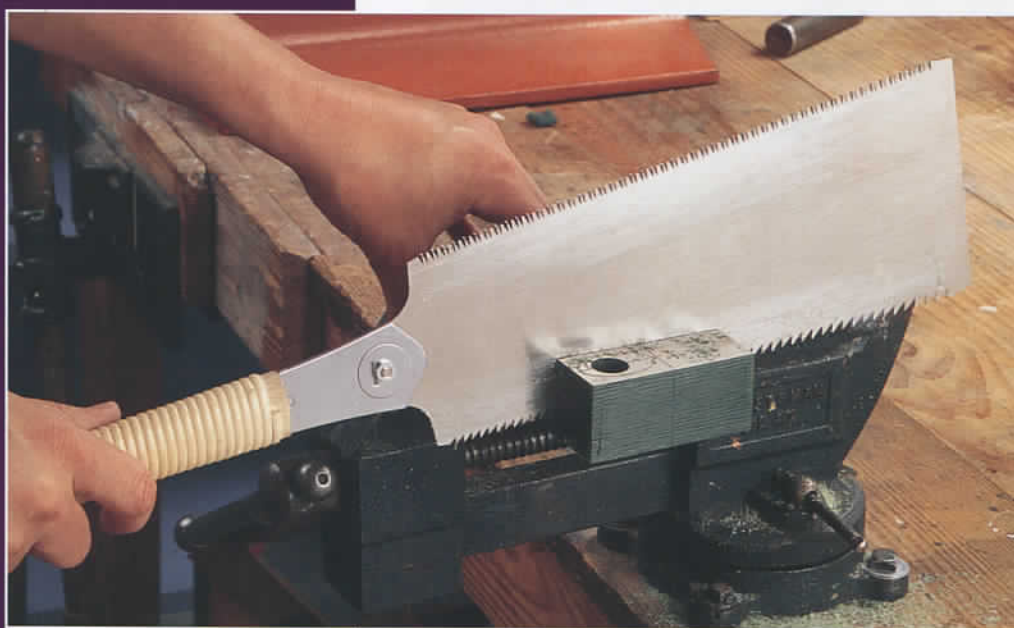
2 I cut the block of wax with a Japanese wood-working saw, but this can also be done with a band saw, scroll saw, or jeweler's saw.
