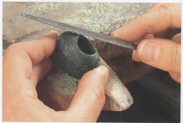
6 The wax ring was further refined with a victory file.
