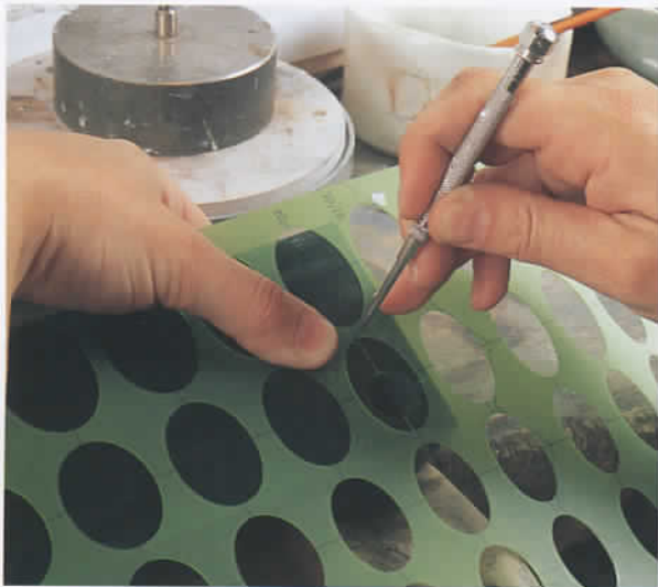
3 The shape of the ring was mapped out with a scribe and templates.
